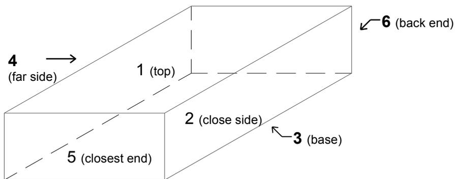
*Package Orientation Definition from AS 2582.1-2003 (isometric view)*
